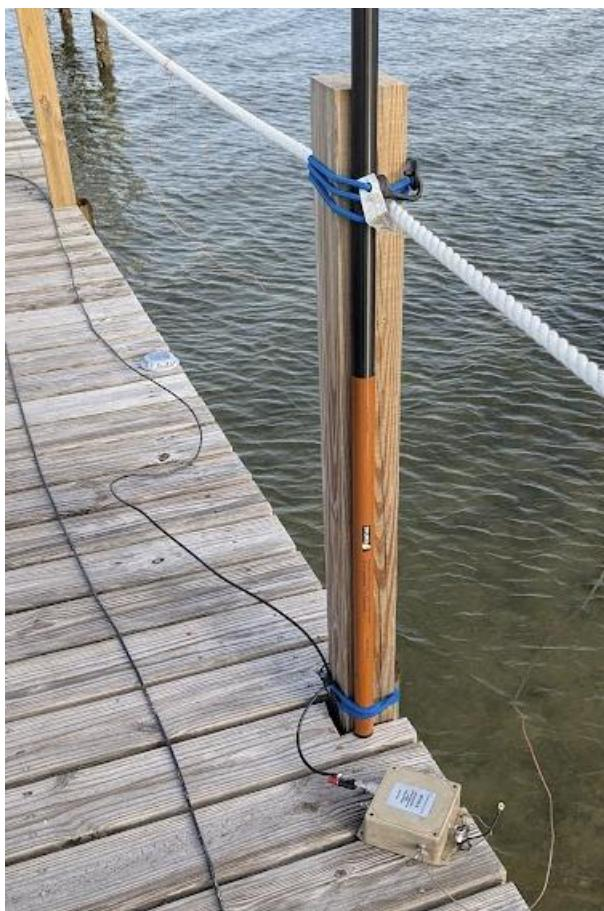
Later, I tried to set up a 40-10 endfed antenna with a matching box by [myantennas.com](#). Something was intermittent. First the box was not tight and had a water damage, with some connections loose. Second, the coax had a bad connector and pulled off as in the picture above.
