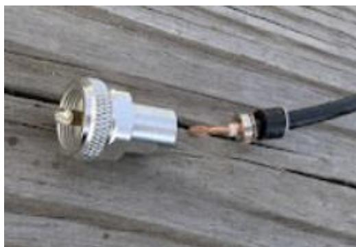
Later tests revealed that while the PL259 connector was soldered, the center conductor was not.
