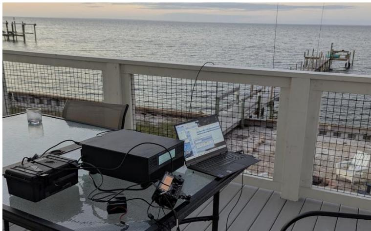
For transmit, the setup included KX3 with a very good receiver and Expert 1.3k-fa amp with a low power mod so that it could be driven to > 1 KW with 5W.
