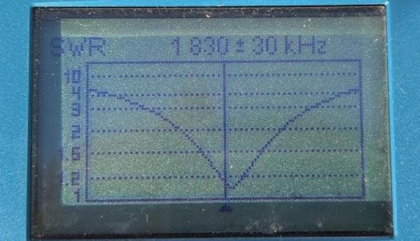
resistance at resonance was only 20 Ohm. For a perfect match, I removed a few turns from the transformer and then the minimum SWR was close to 1:1.
