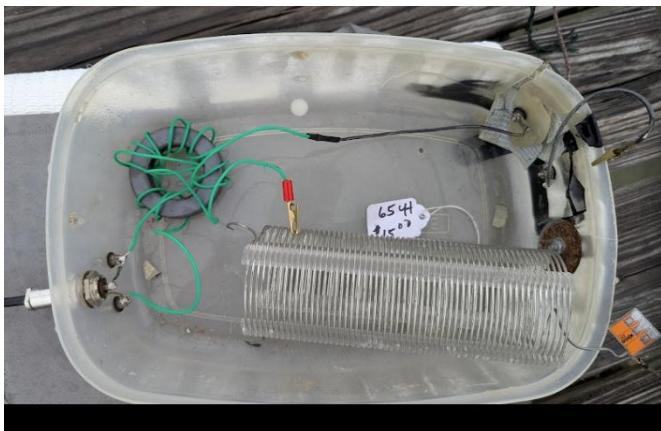
An old matching box consisted of a transformer on a 240-61 ferrite and a 75 microH coil with a tap.
