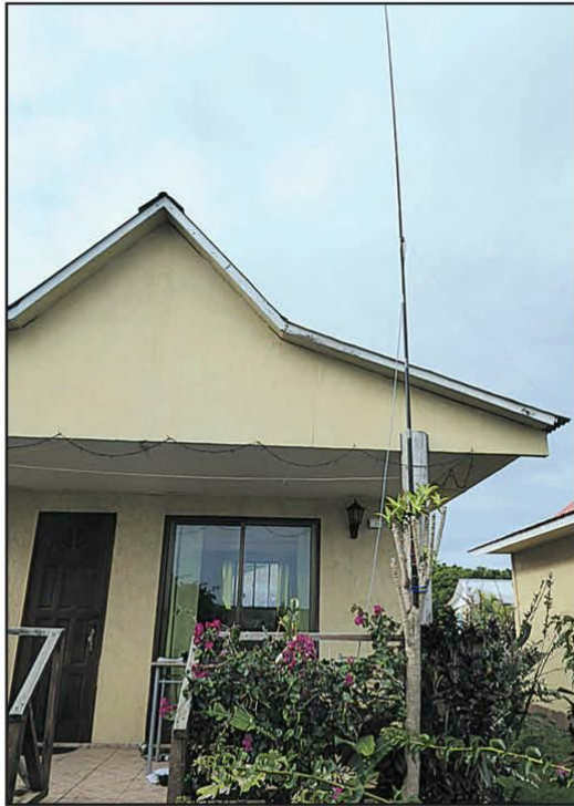
Photo E. A 15-meter vertical with drooping radials was set up in front of the house for comparison with the EFHW.
