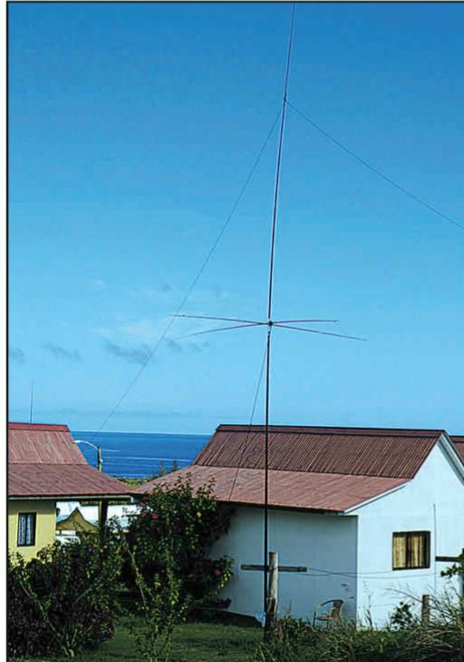
Photo D. The end-fed half-wave set up as an inverted-V atop a 40-foot (12-meter) Spiderpole.
